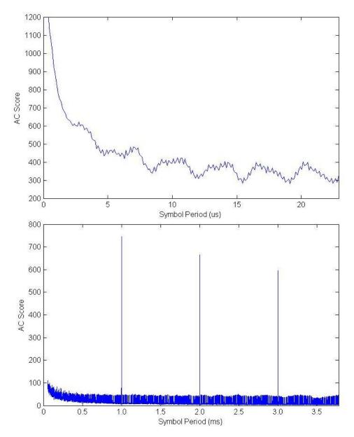
Figure 10: Comparison of SWAC plots for a non-spread BPSK modulation from the GOES satellite (top) and a spread BPSK modulation from a GPS satellite (bottom)
