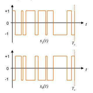
Figure 4: An illustrative spread-spectrum BPSK signal set – an example of a highdimensionality binary antipodal alphabet
