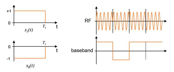
Figure 3: BPSK signal set, with example waveforms at RF and baseband
