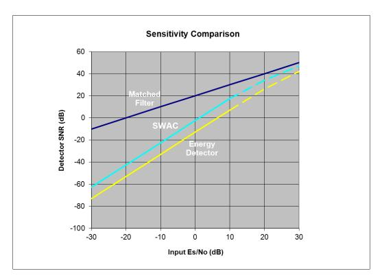
Figure 13: Sensitivity comparison of three detector types, assuming an antipodal spreadspectrum BPSK signal in Gaussian noise (symbol rate 1 symbol/s, spreading factor 500, sampling rate (=noise bandwidth) 1kHz, measurement interval 100 seconds (M=100))
