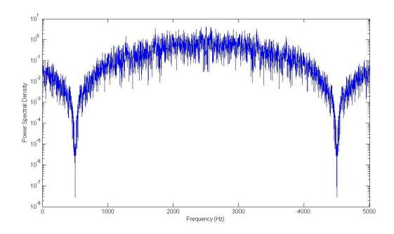
Figure 5: PSD for an illustrative antipodal spread-spectrum BPSK signal (2 symbol/s, 1000 chips/symbol, no noise)
