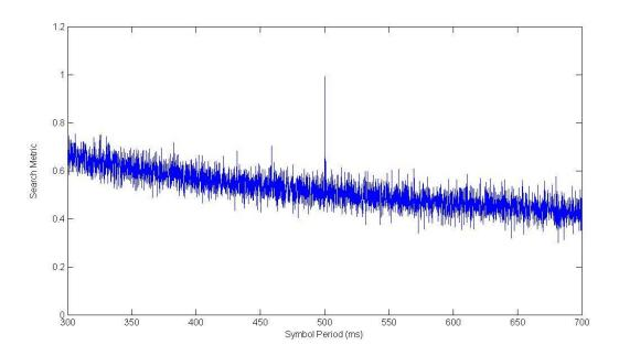
Figure 8: SWAC output as a function of assumed symbol period  $\tau$ , with the waveform of Figure 7 as input
