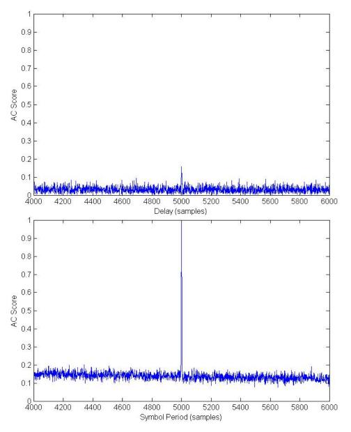
Figure 11: Comparison of conventional autocorrelation (top) with SWAC (bottom) for a spread-spectrum BPSK signal embedded in Gaussian noise with SNR of -10 dB
