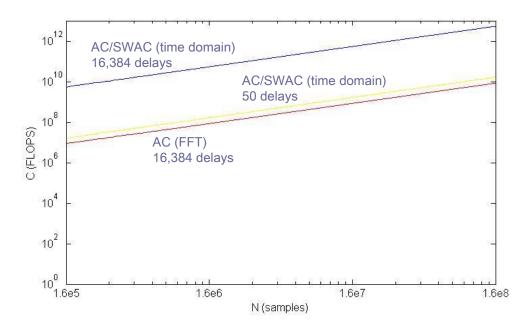
Figure 17: Computational complexity versus N for different autocorrelation-based algorithms
