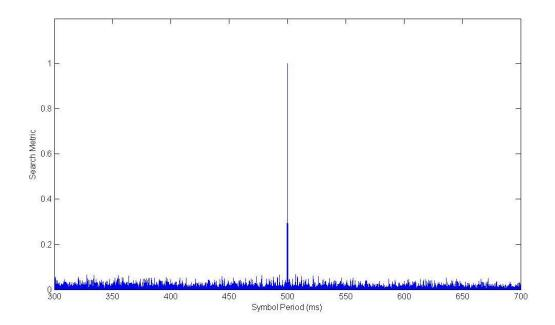
Figure 6: SWAC output as a function of assumed symbol period  $\tau$ , with the waveform of Figure 5 as input
