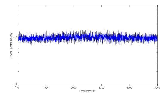
Figure 7: PSD for the illustrative signal of Figure 5 embedded in Gaussian noise (white across the measurement bandwidth)
