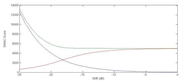
Figure 12: Variation in SWAC score versus input SNR for an illustrative spread-spectrum input signal in Gaussian noise. The green curve is for [signal+noise], the blue curve is for [noise only] and the red curve is the difference between green and blue.
