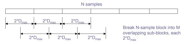
Figure 14: Overlapped sub-blocks for FFT based computation of autocorrelation
