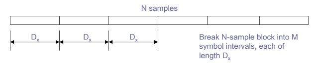
Figure 16: Partitioning into sub-blocks for SWAC processing
