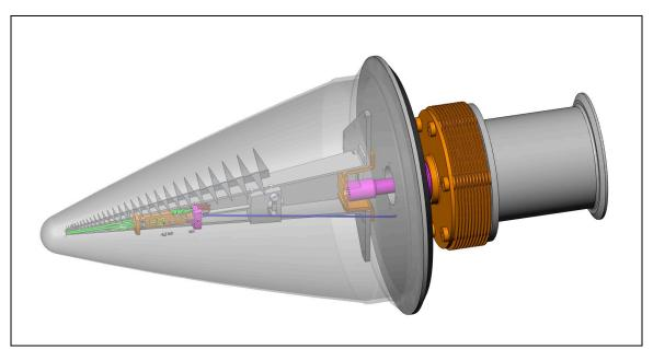
Figure 4- Details of the feed within the dewar. The glass is very thin near the tip and much heavier near the back end. It is largely transparent to the feed radio waves.
