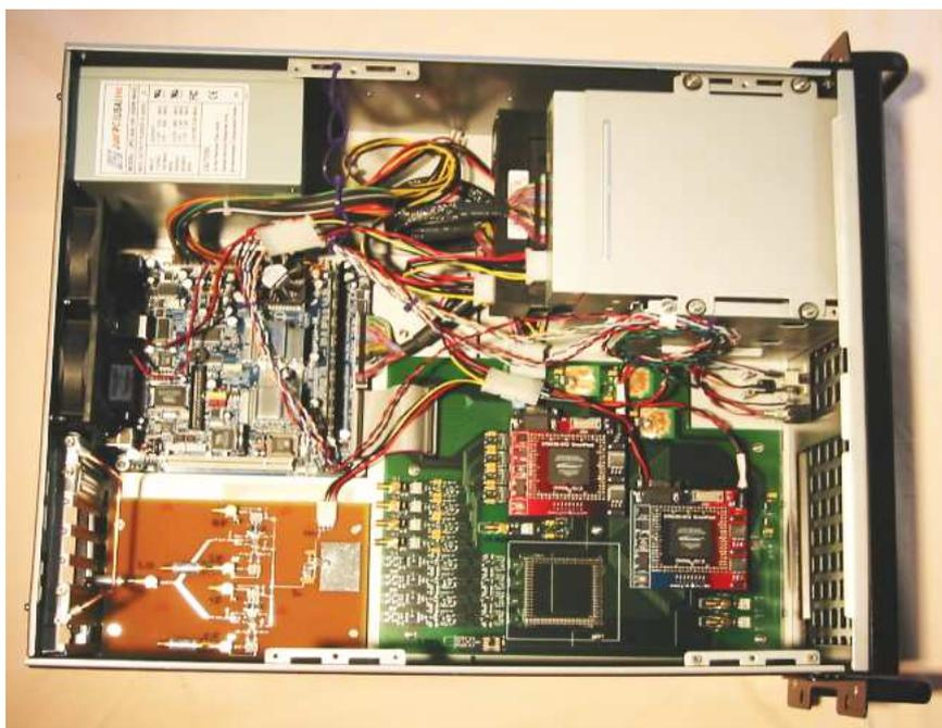
Figure 1: beamformer assembled in 4U server rack-mount case
