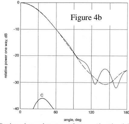
Copolar and crosspolar patterns of a waveguide with a choke
