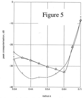
Peak crosspolarisation of a circular waveguide
