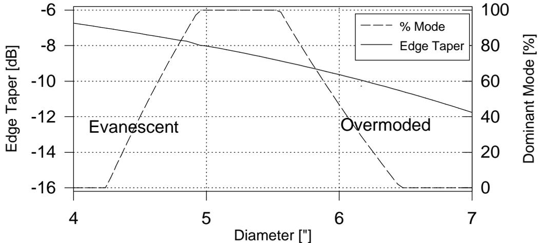
The choke (or scalar ring) was designed based on experience with C-band TVRO feeds. Chokes are typically used to improve the match, gain, cross-polarization and pattern symmetry. A good reference for chokes is Olver *et al.* 1994, and results from that text will be summarized. In addition, the choke provides a convenient mount point for the feed, both in interfacing with the leg supports and in providing free parameters to optimize performance. Figure 2 shows a schematic of the feed assembly.
