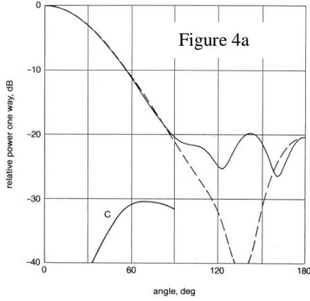
Copolar and crosspolar patterns of a waveguide without a choke
