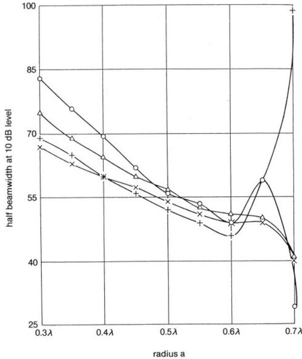
Figure 3 10 dB beam angles for a circular waveguide
