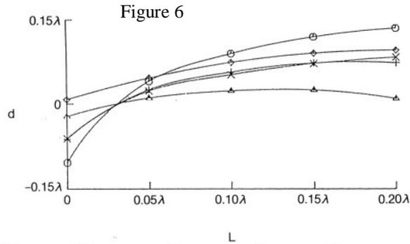
Distance of phase centres from waveguide open end for geometry of Figure 7
