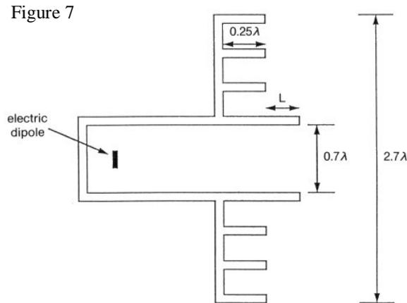
It is suggested to mount one feed as suggested above, point the dish at an L-band geostationary satellite, and move both the choke relative to the dish and the feed relative to the choke, until maximum gain is achieved. Note that most of the L-band downlinks are right-hand circularly polarized, so orientation of the feed will not be an issue. Additionally, it would be a good idea to make sure the maximum gain point is similar for both linear polarizations.
