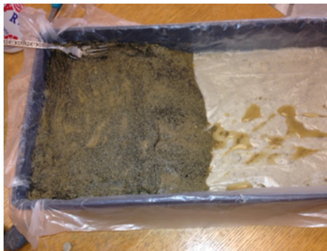
Prop up the sand-filled end 10 degrees with foam slices.
