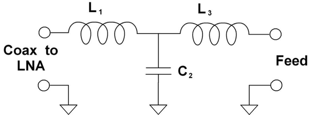
Figure 8: The low pass filter joining coax to feed.
