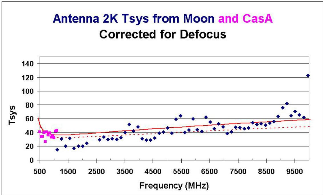
Figure 2:  $T_{\text{sys}}$  measurements corrected for defocus but not for the variation in feed gain.
