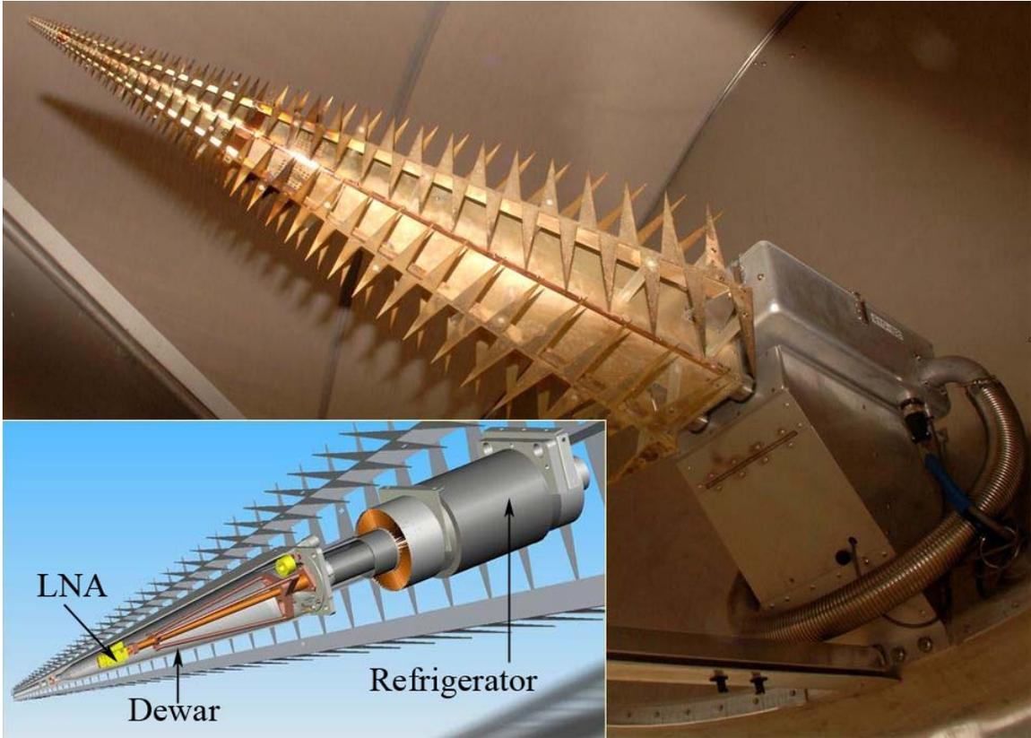
Figure 1: above: A photograph of the ATA feed mounted in an antenna. below: a drawing with the pyramid removed, showing the LNA, dewar, and refrigerator.
