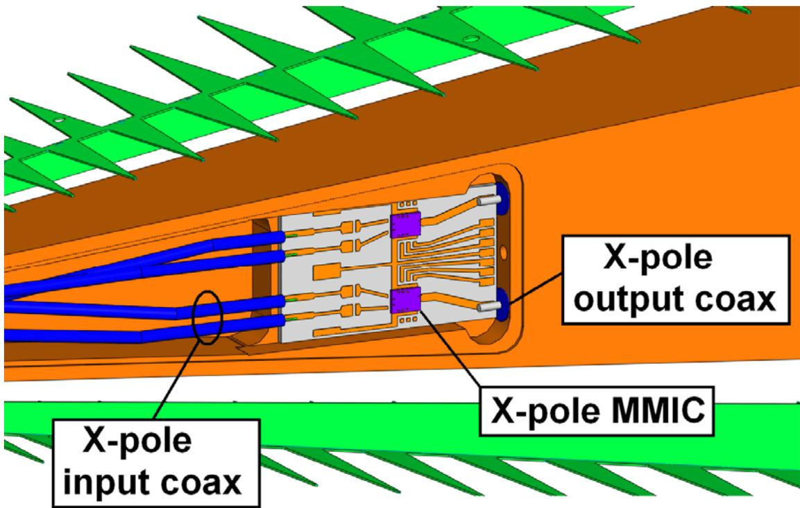
Figure 7: Detail of the mimic chip location and input cables.
