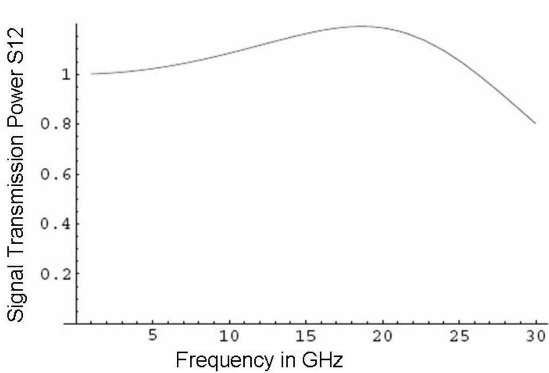
Figure 9: Frequency response of the low pass filter connecting coax and LNA to feed antenna.
