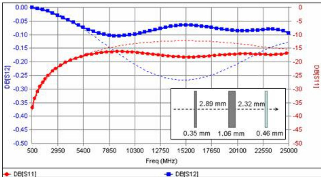
With 2 layers of Teflon anti-reflection coating
