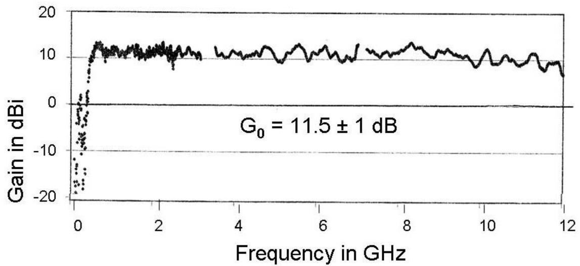
Figure 3: Accurate (~1%) log-periodic feed gain measurements.
