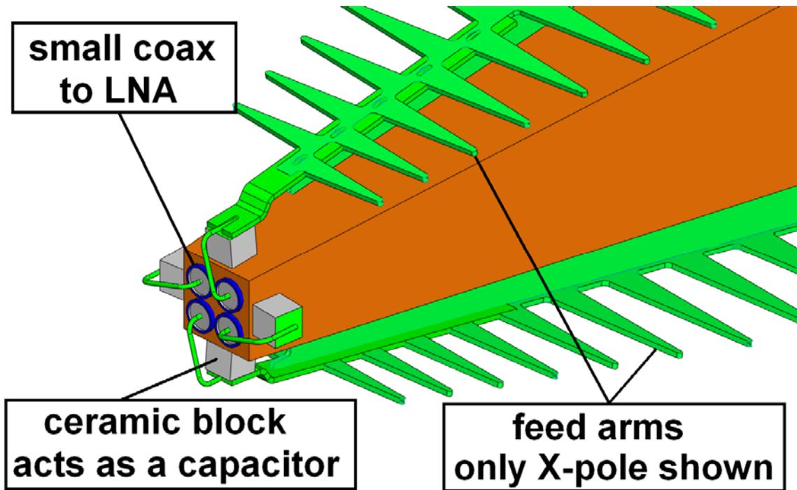
Figure 5: New feed conception; Coax lines are .03 inch diameter; Caps are .03 inch cubes
