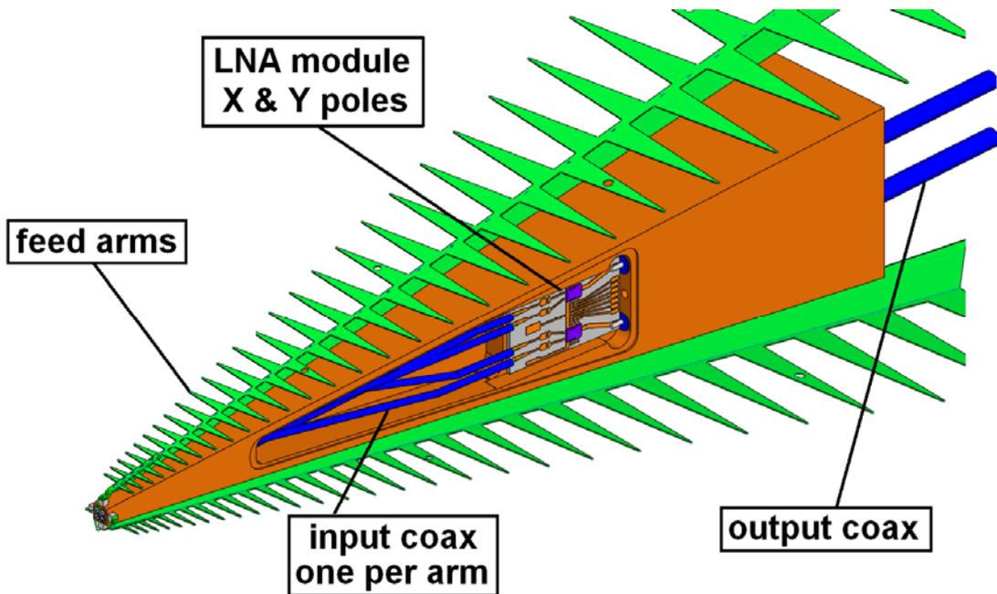
Figure 6: Planned feed showing location of coax cables and LNA module.
