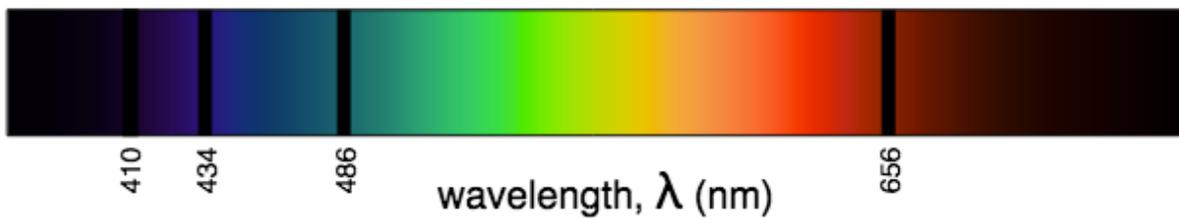
A cool, transparent gas in front of a hot, opaque body produces an absorption (dark-line) spectrum.
