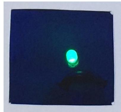
3) *Elaborate:* Distribute spectroscopes, blue filter, green and white LEDs, batteries, and pencils or crayons. (The spectroscpe will show that green LED light is really made up of green, as well as some blue light.)
