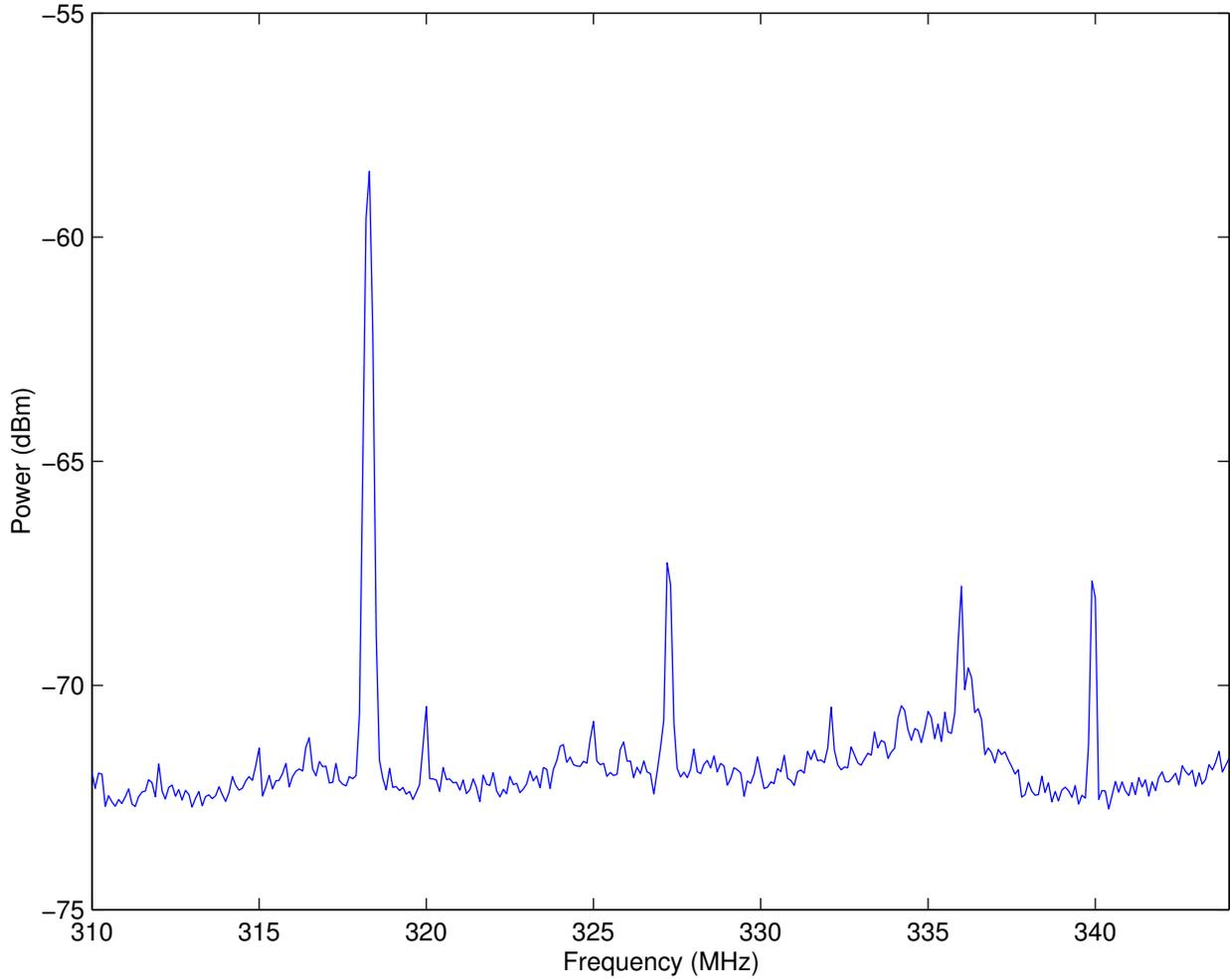
Fig. 6.— RFI spectrum captured on 11 September 2002 at Hat Creek. This is the mean of 35 2-minute integrations. The feature at 327 MHz is present in each integration. The feature also appeared in each of 12 1-hour integrations on the same day. The feature was not apparent in 5-minute integrations on 25 September 2001.
