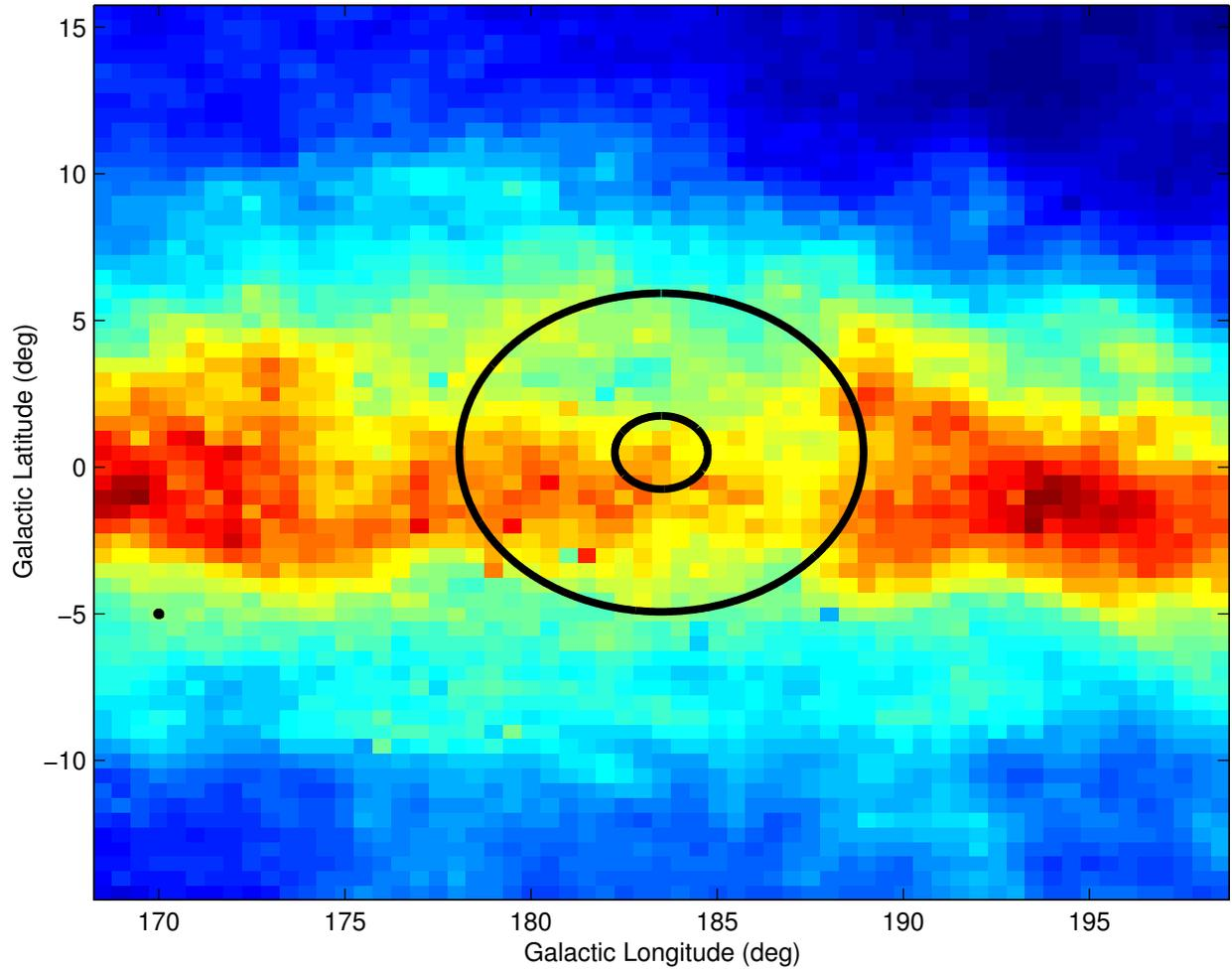
Fig. 2.— Map of HI brightness temperature integrated over velocity in the Galactic anti-center from the Leiden-Dwingeloo survey. The ATA primary beams at 21 cm and 90 cm are shown. The 90 cm synthesized beam for the ATA-32 is also shown.
