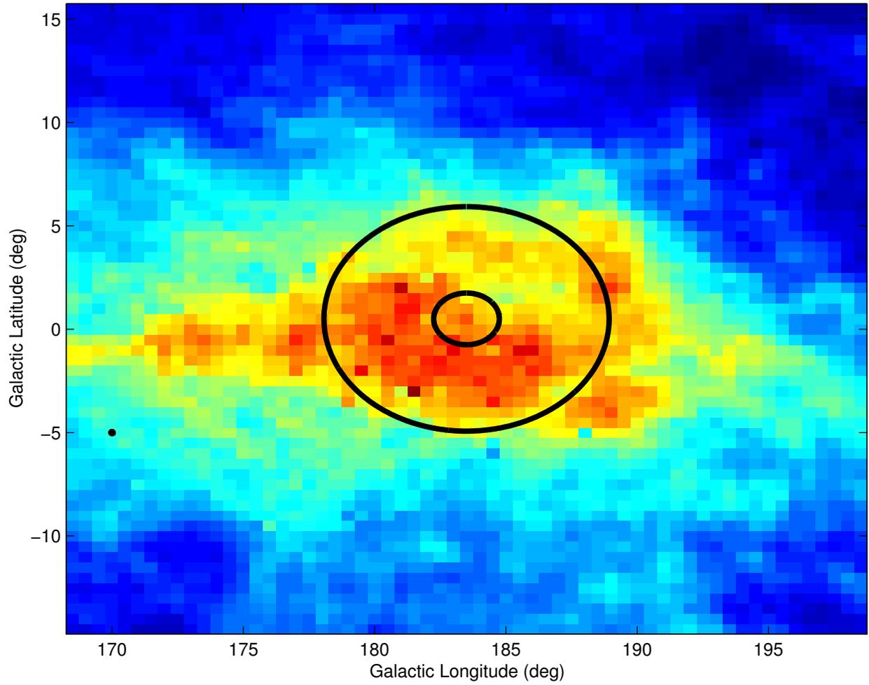
Fig. 1.— Map of HI brightness temperature at zero LSR in the Galactic anti-center from the Leiden-Dwingeloo survey. The ATA primary beams at 21 cm and 90 cm are shown. The 90 cm synthesized beam for the ATA-32 is also shown.
