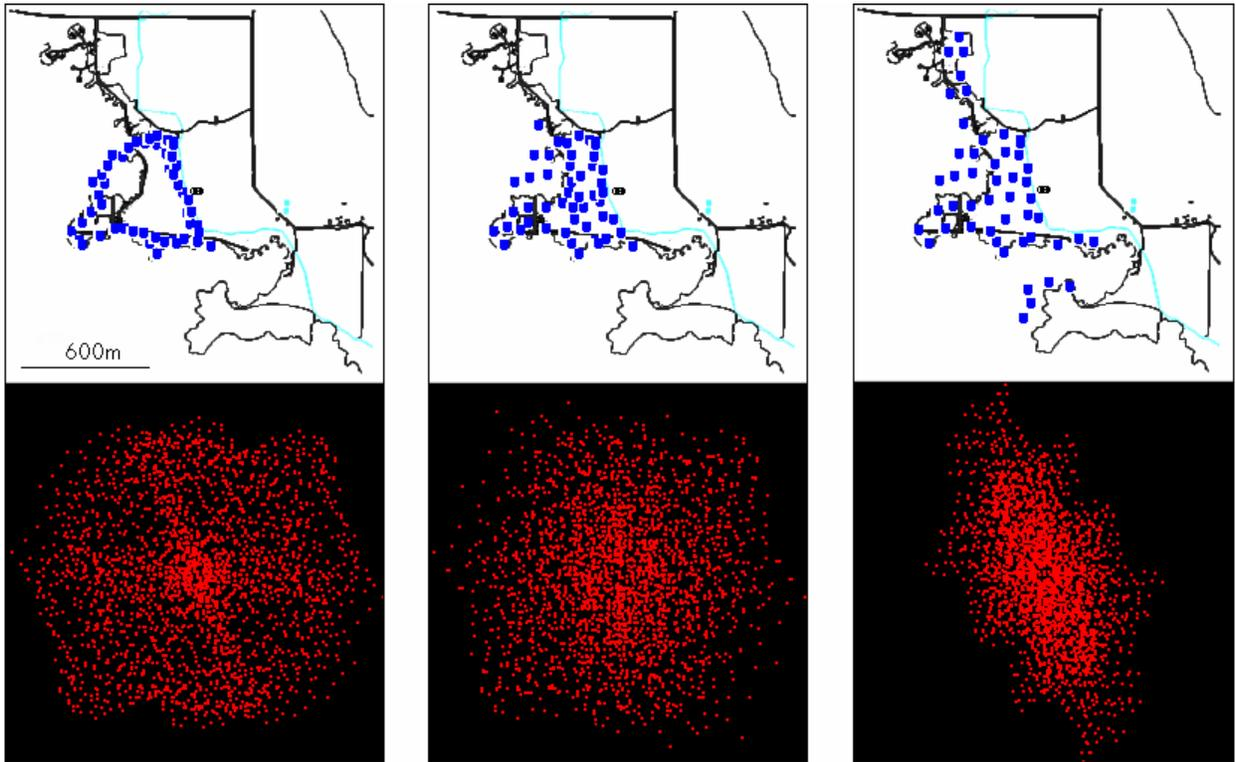
Fig. 2.— Three sample configurations, from left to right: ‘compact open’, ‘compact filled’, and ‘extended’. In each case the antenna configuration is shown overlaid on a representation of the Hat Creek site, together with snapshot ( $\delta = 30^\circ$ )  $u-v$  coverage (not to scale).
