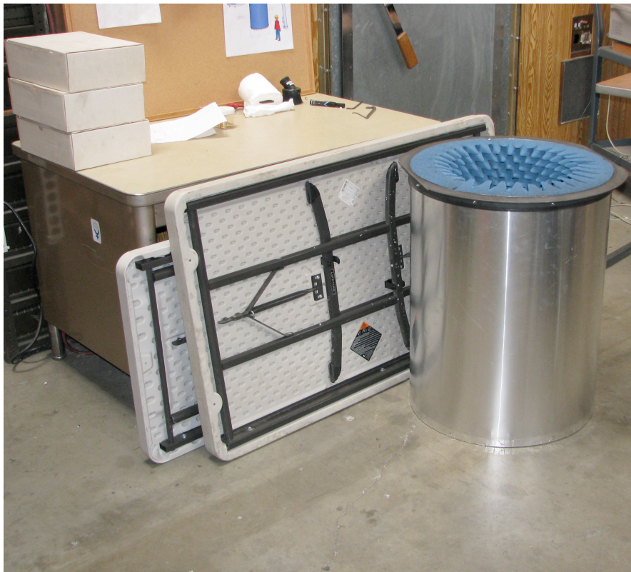
Figure 13 is a photograph of the hot load. The cylinder with the inner absorber is placed over the feed to provide the known ambient reference. Its length is long enough to insure that all parts of the feed are covered. Its physical temperature is directly measured with a thermometer ( = 304\text{K} ). The absorbing material was tested and showed that its two way transmission is less than -44\text{ dB} at all relevant frequencies. It should be an essentially perfect black body at its measured temperature.
