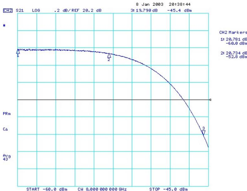
Figure 15. Gain vs. input power for the PAM (s/n 2) + fiberoptic link.
