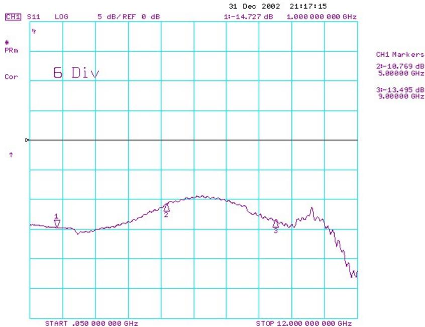
Figure 6. S11 at the RF input (GPO connector) on the NEC laser module.
