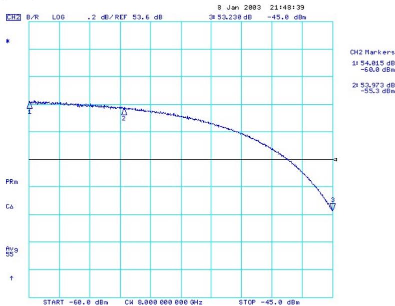
Figure 13. Gain of PAM s/n 2 at 8 GHz, vs. input power level, measured with the 8722D network analyzer.
