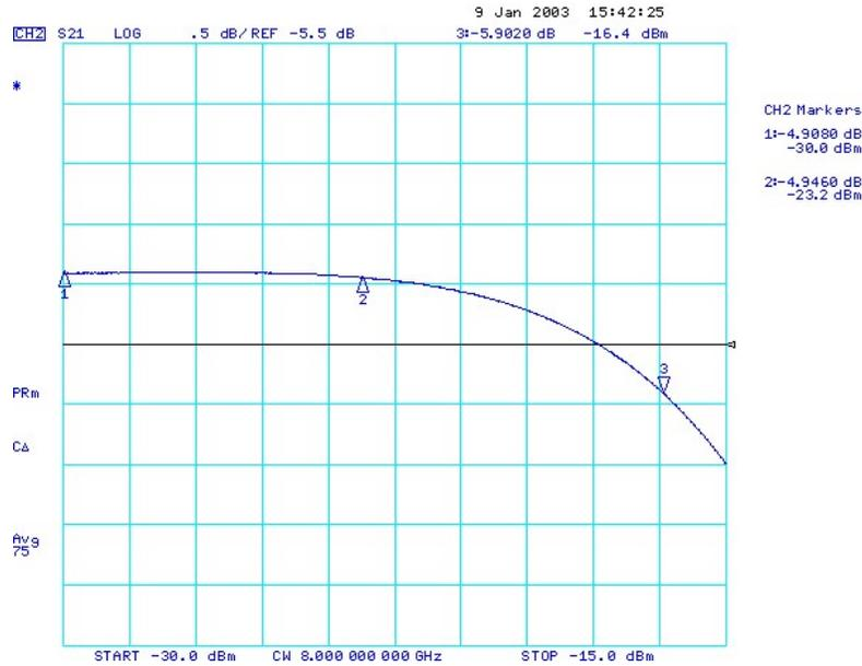
Figure 14. Gain of link alone, vs input power. The link was preceded by a JCA amplifier with  $28$  dB gain at  $8$  GHz, so the actual sweep range is  $-2$  to  $+13$  dBm.
