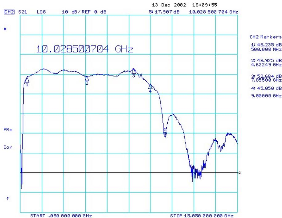
Figure 1. S21 of PAM s/n 3, measured with an 8722D network analyzer. The attenuators in the module were set to 0 dB for this measurement.
